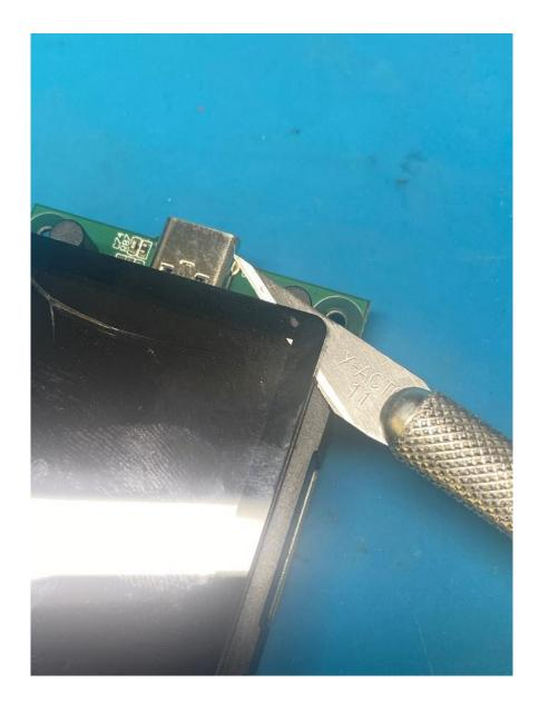
Once removed, carefully take the new screen cover and place it as accurately as possible since it will need to fit back into the chassis.
