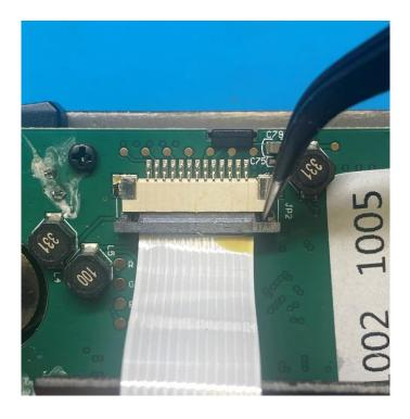
Remove the 4 silver screws from the LCD board and carefully lift the board up.
